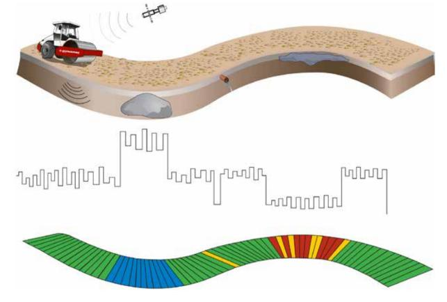
Continous Compaction Control using accelerometer based on stiffness readings allows the roller operator to "see" below the surface.
