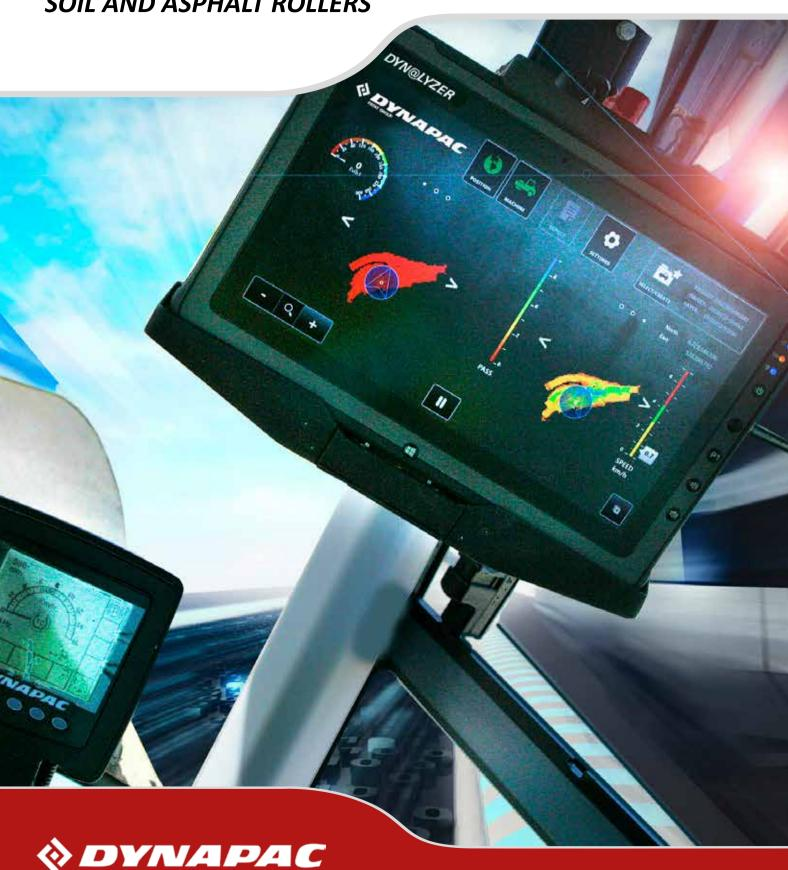
DYNAPAC'S EXPERIENCE in Continuous Compaction Control (CCC) or Intelligent Compaction (IC) dates back to the late 70s. Since then we have been able to offer our customers the opportunity to control the compaction work in real time and to document the completed work for improved quality control.
