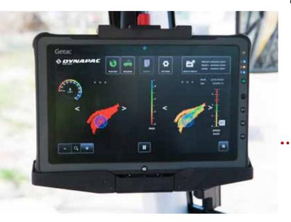
The on-board display shows a map of the recorded data to the operator; in this case passes and the asphalt temperature.
