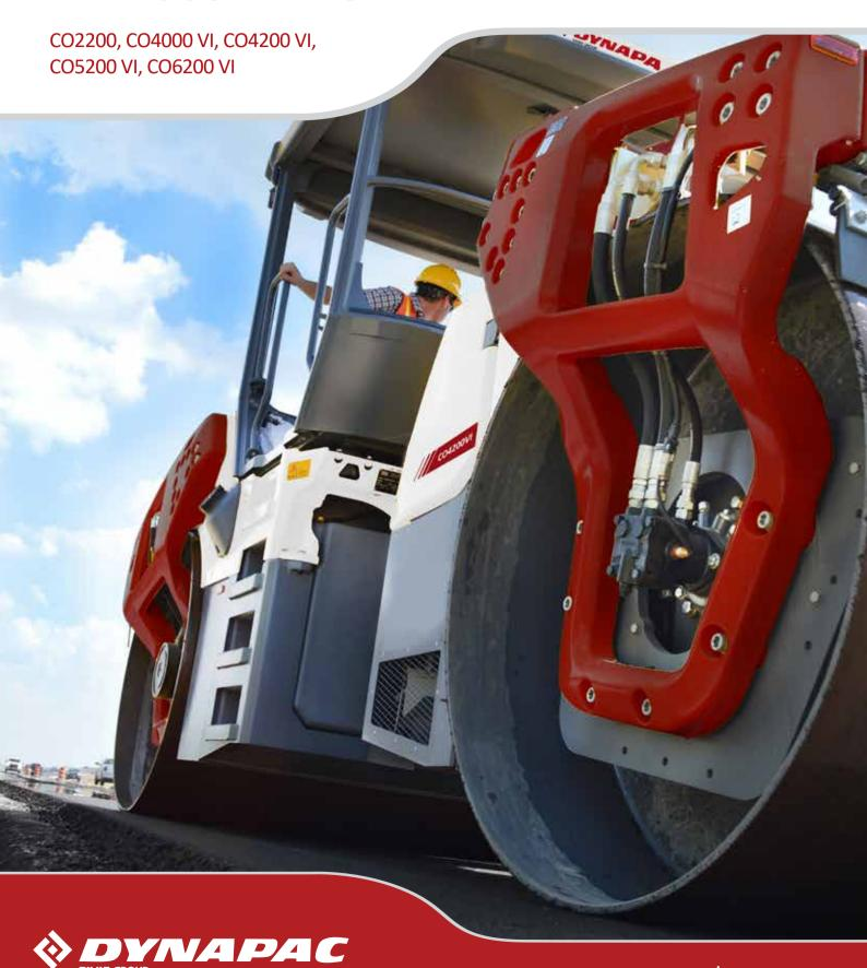
Together with the high vibration frequency concept on the large asphalt tandem rollers Dynapac also offers the oscillation concept. Meeting the special needs of the oscillation compaction concept, Dynapac has focused on **wear resistance and service-ability** in order to supply a long lasting and user friendly solution.
